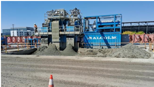
Desanders being used to remove sand and other particles from drilling fluids.
