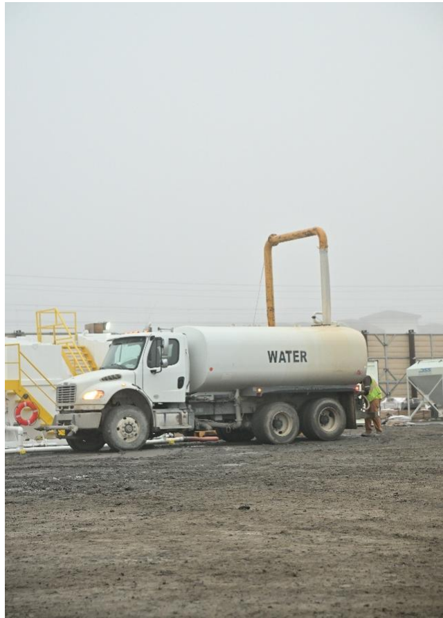
A water truck is refilled onsite to support dust management and keep drilling and excavation running safely and smoothly.
