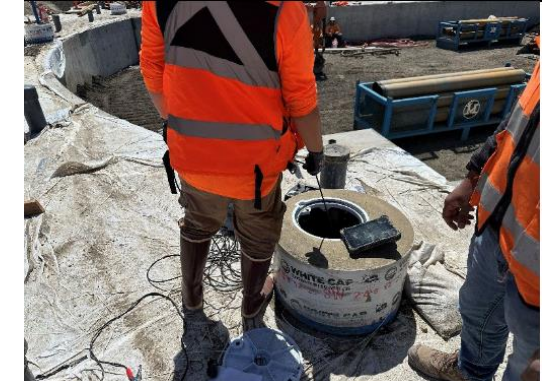
Manual Reading of Inclinometer
